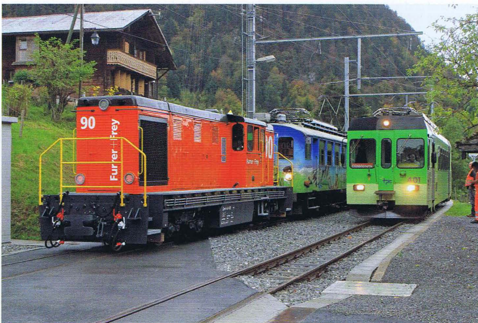
Above: Load test of adhesion diesel locomotive Gmf 4/4 90 hauling the MGB 50 t rack motor car Deh 4/4 23 in 70% grade up from Nättschen to Oberalppass (photo: J. Blaser, 7 October 2014).
