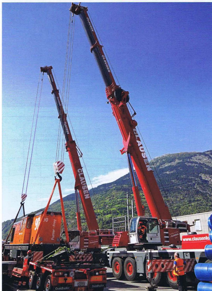
Left: Transferring Gmf 4/4 90 from the railway wagon onto the low-loader semitrailer with two truck-mounted cranes in loading/unloading siding H25 at Brig station (photo: P. Gerber, 29 September 2014).
