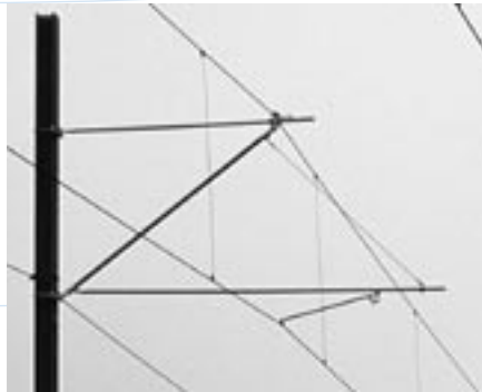
Cantilever geometry with horizontal adjustment
